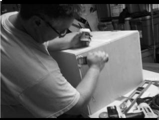
We wanted the wood for the box to be both light and strong. We needed the box to not weigh too much, but it had to be sturdy for the performances. In this picture, Don is working to securely build the box. He used nails, screws, wood glue, putty, and brackets to make the box a strong structure.
